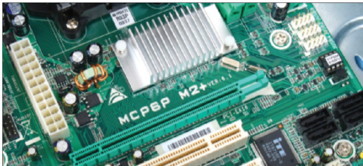
Figure 3-39 The motherboard brand and model are imprinted somewhere on the board Courtesy: Course Technology/Cengage Learning
