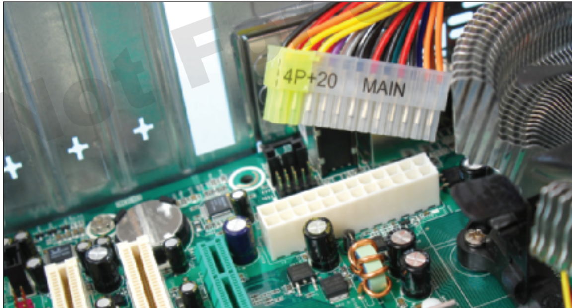
Figure 3-49 The 24-pin connector supplies power to the motherboard Courtesy: Course Technology/Cengage Learning
