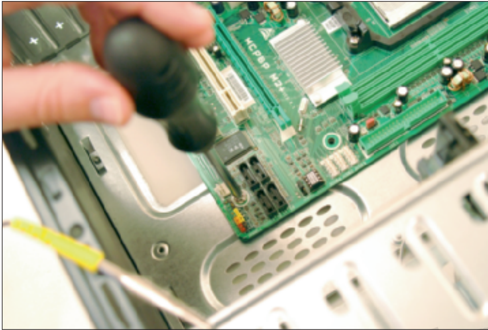
Figure 3-48 Use one screw in each screw hole on the motherboard Courtesy: Course Technology/Cengage Learning
