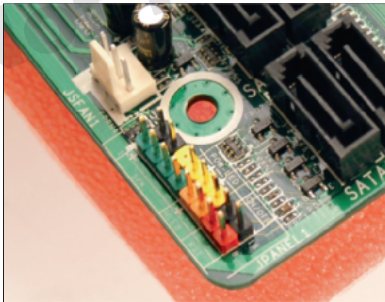
Figure 3-53 Front panel header uses color-coded pins Courtesy: Course Technology/Cengage Learning
