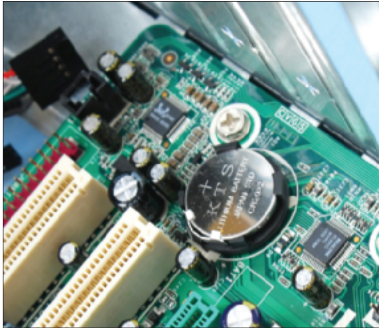
Figure 3-30 The coin-cell battery powers CMOS RAM when the system is turned off Courtesy: Course Technology/Cengage Learning
